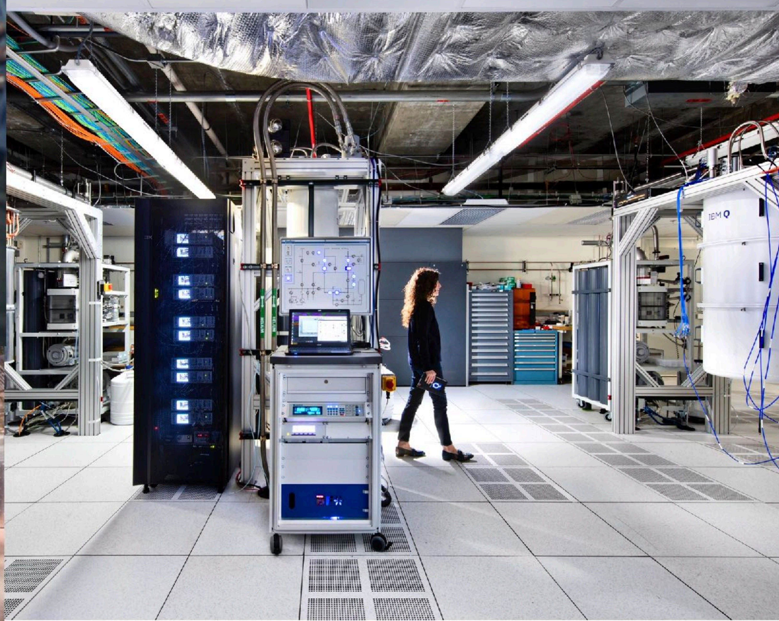
IBM's quantum computing center at the Thomas J. Watson Research Center in Yorktown Heights, New York, holds quantum computers in large cryogenic tanks (far right) that are cooled to a fraction of a degree above absolute zero.
